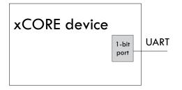
Figure 3: UART half duplex connection
