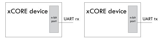
Figure 2: UART Rx and Tx connections
